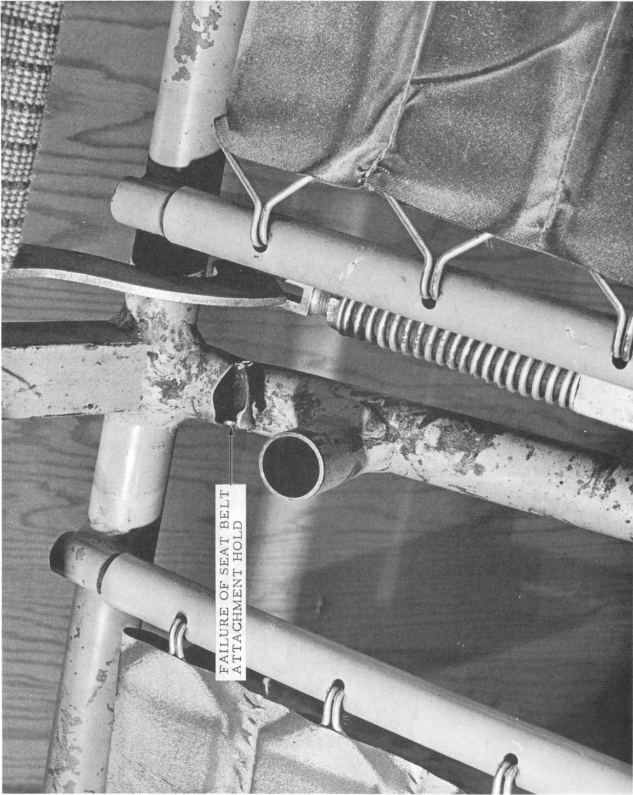
FIG. 3-8 RIGHT BOTTOM SUPPORT - SEAT A-5 AFTER TEST NO. 71
