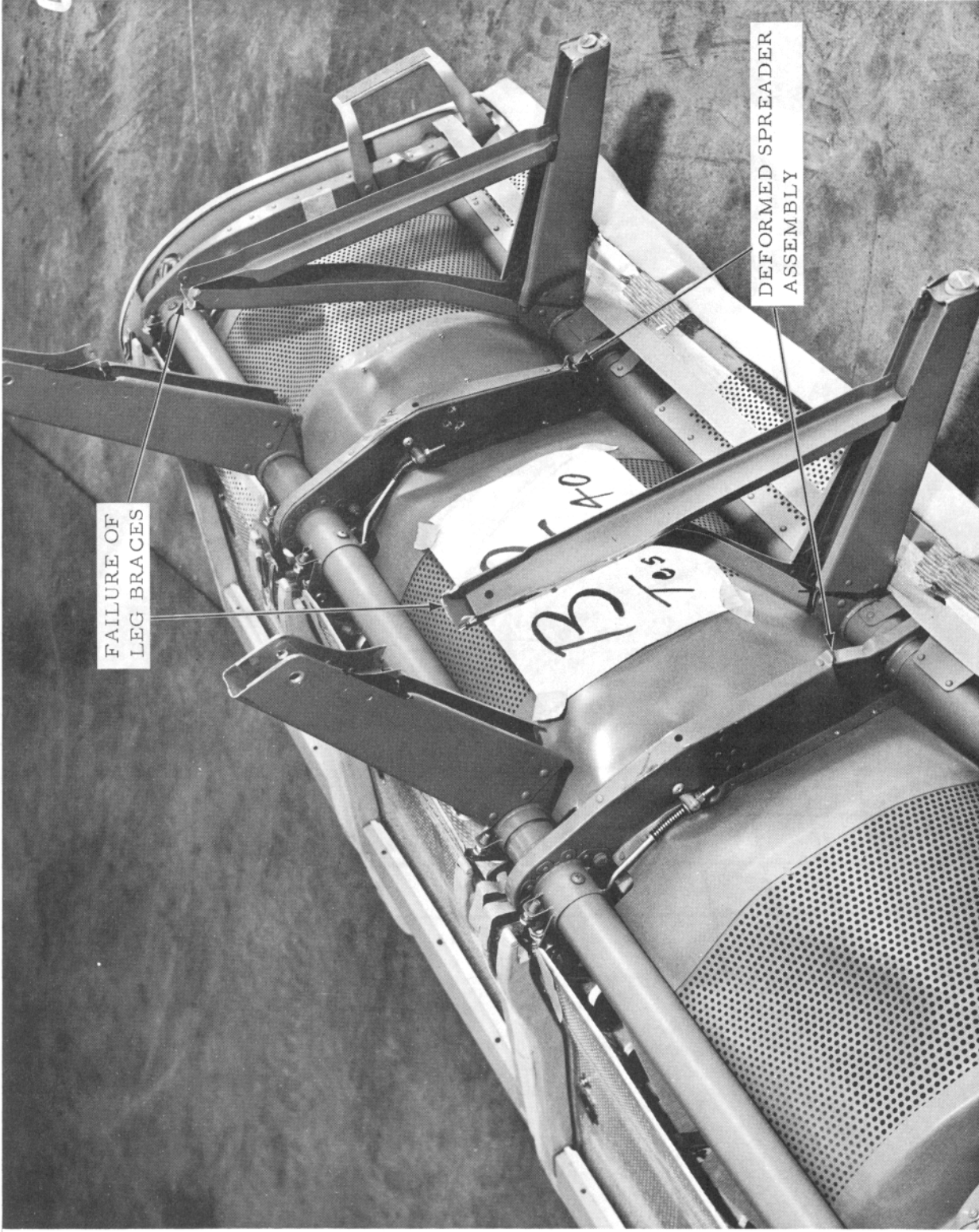
FIG. 3-14 BOTTOM VIEW OF SEAT B-2 AFTER TEST NO. 40
