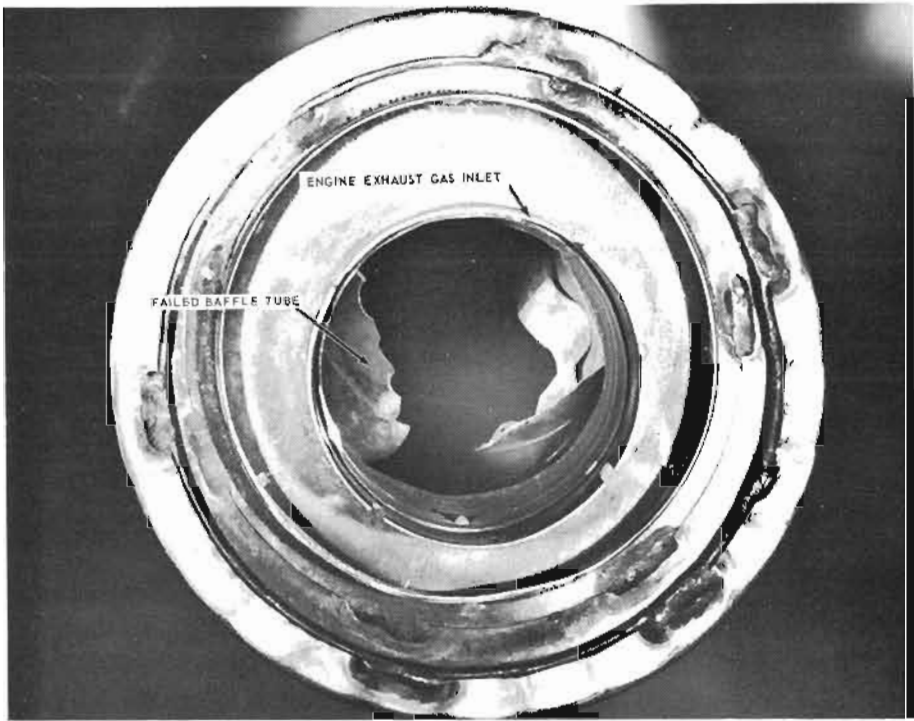
FIG. 1.5 FAILED MUFFLER BAFFLE TUBE
