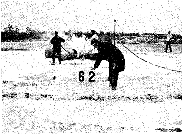
(1) "FLUOROPROTEIN" FOAM ALONE FOAM DISCHARGE RATE - 400 GAL/MIN
