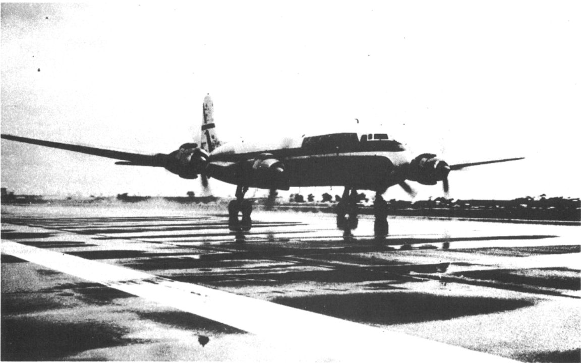
FIGURE 10. DC-7 TEST AIRCRAFT DURING MAXIMUM WET TESTS
