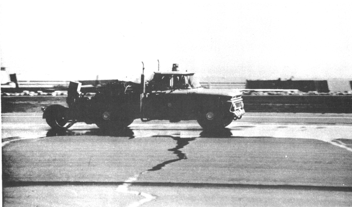
FIGURE 7. FAA VARIABLE SLIP RUNWAY FRICTION TESTER
