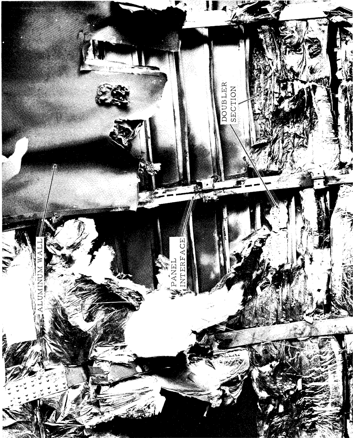
FIGURE 18 - BURNED INSULATION ABOVE DOUBLER SECTION
