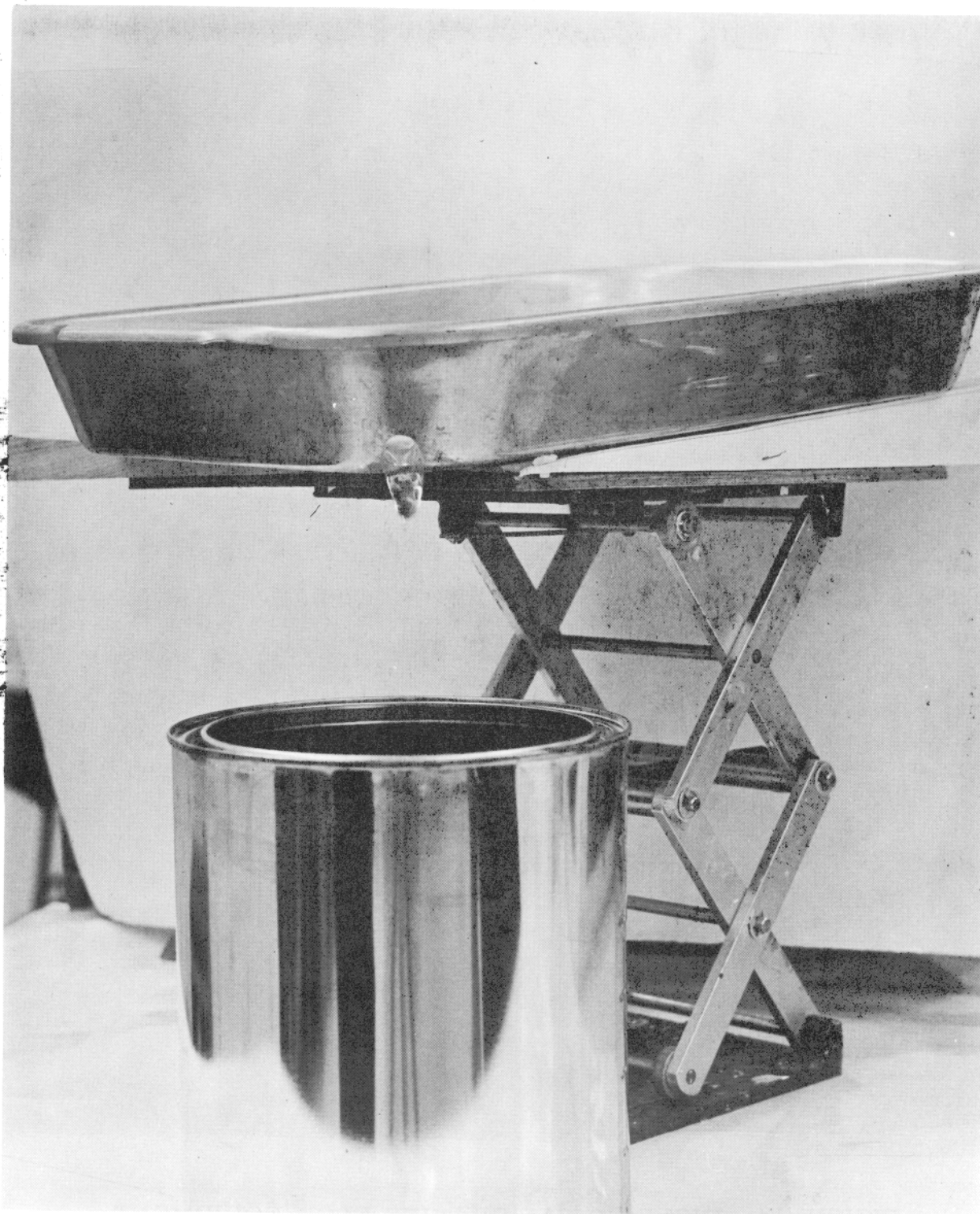
FIGURE 13. INCLINED PAN GRAVITY FLOW EQUIPMENT (FUEL COMPOSITION 2-10-0; THICK GEL)
