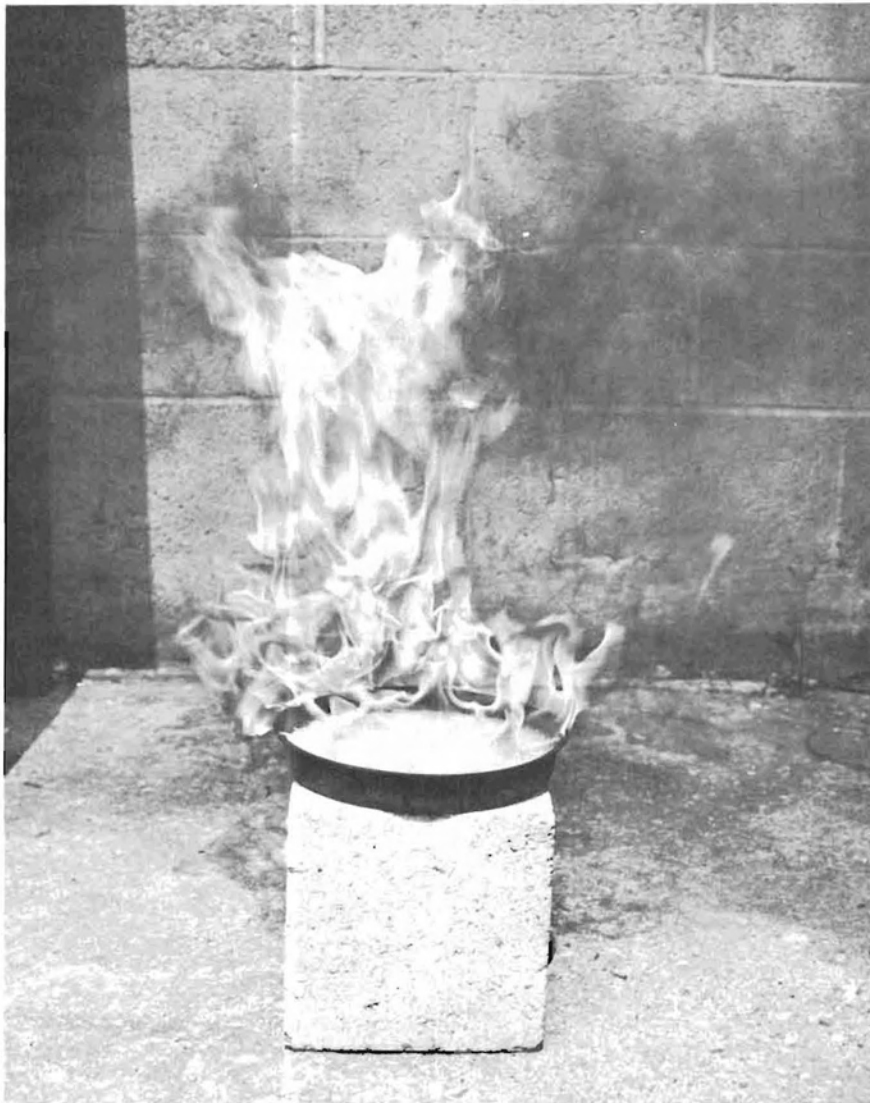
FIGURE 2-5 - TRAY CONTAINING EMULSIFIED FUEL DURING BURNING RATE TEST
