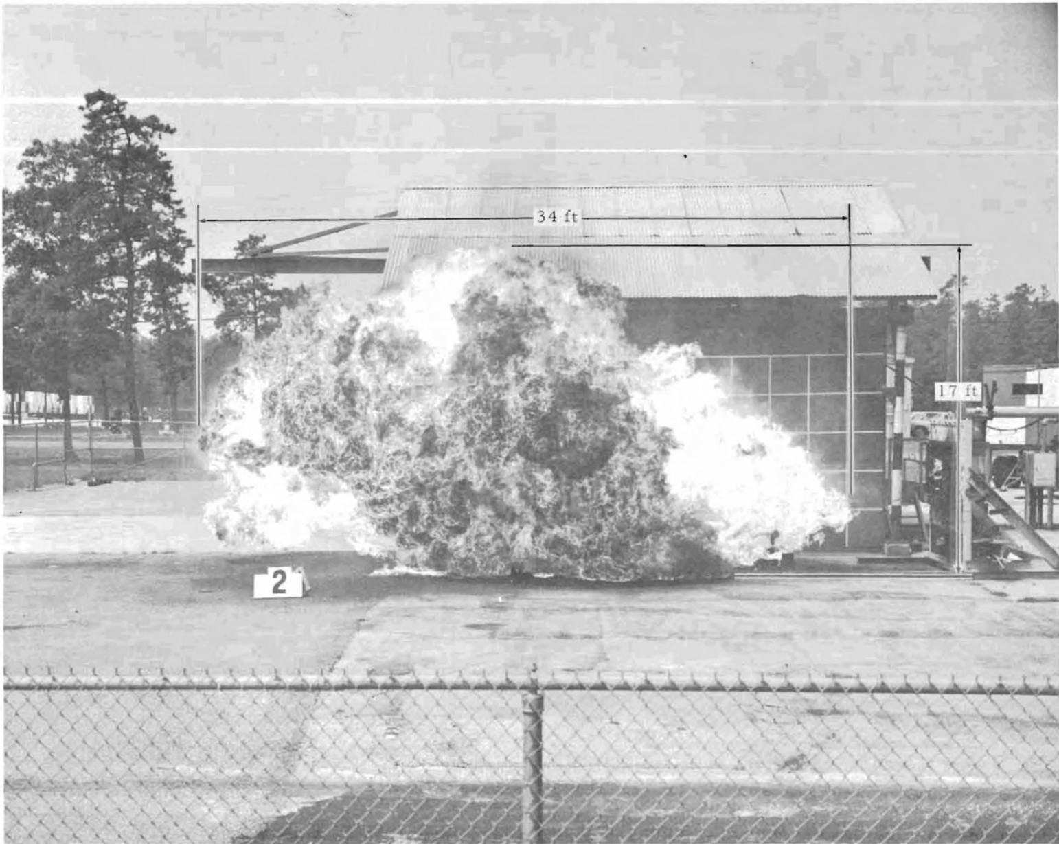
FIGURE 5 - JET A FUEL-MIST EXPOSED TO OPEN FLAMES - AIR GUN TEST
