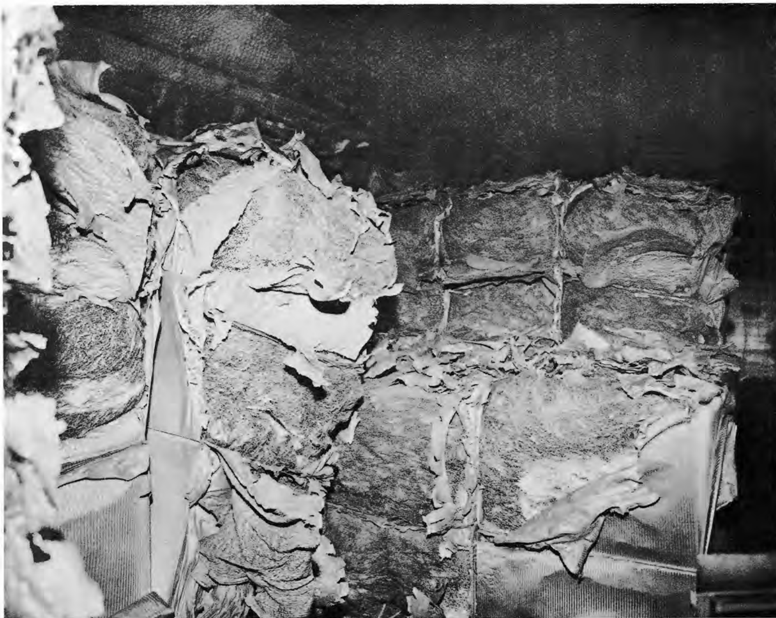
FIGURE 12 - CARGO LOADED IN CARGO COMPARTMENT IN THE 10-PERCENT CONFIGURATION AFTER AN AIRFLOW-SHUTOFF TEST, LOOKING FROM THE INLET END
