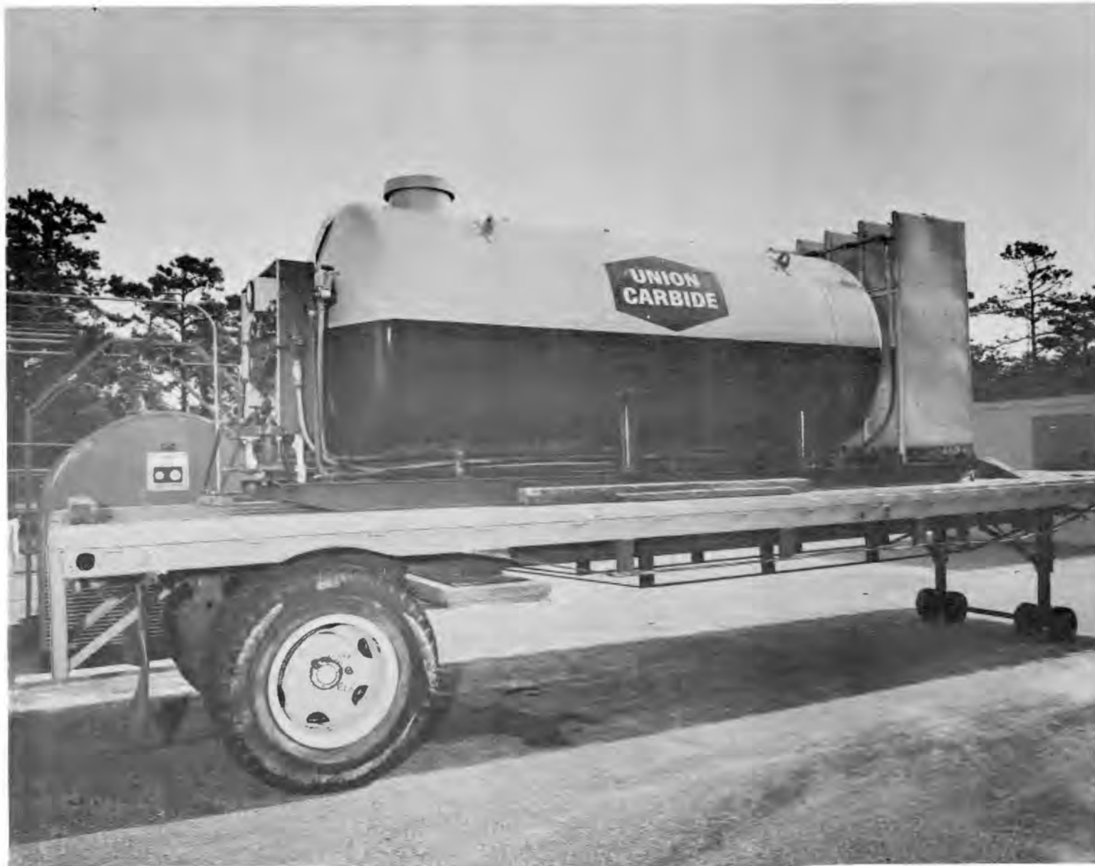
FIGURE 9 - TRAILER CONTAINING LIQUID NITROGEN
