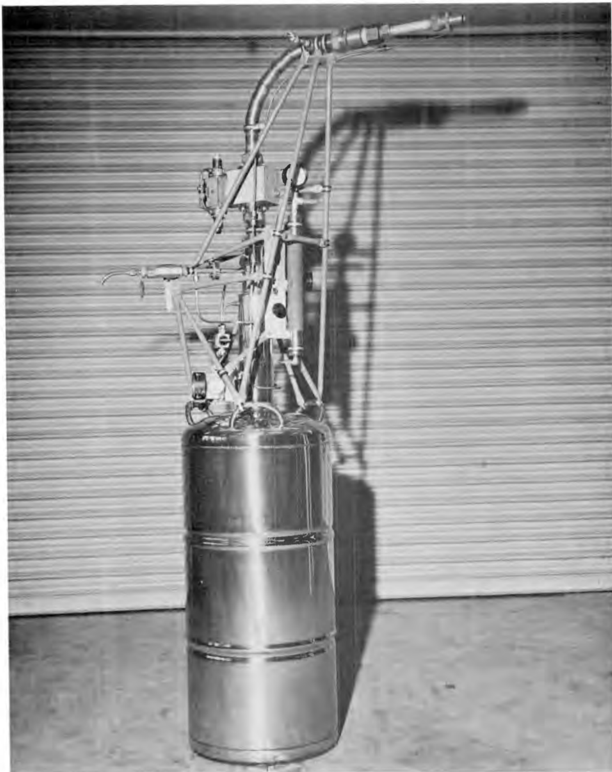
FIGURE 8 - DEWAR USED IN THE LIQUID NITROGEN EXTINGUISHING TESTS
