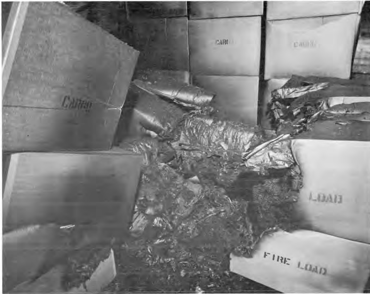
FIGURE 16 - CARGO LOADED IN CARGO COMPARTMENT IN THE 10-PERCENT CONFIGURATION AFTER A BROMOTRIFLUOROMETHANE-EXTINGUISHING TEST, LOOKING FROM THE INLET END
