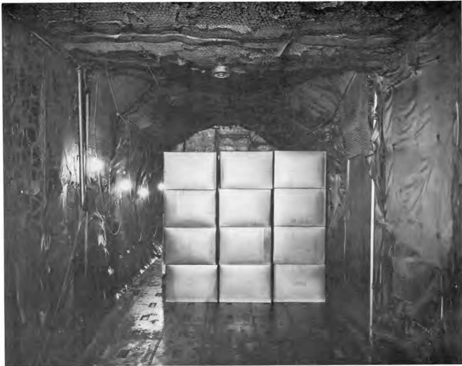
FIGURE 17 - CARGO LOADED IN CARGO COMPARTMENT IN THE 10-PERCENT CONFIGURATION AFTER A BROMOTRIFLUOROMETHANE-EXTINGUISHING TEST, LOOKING FROM THE OUTLET END
