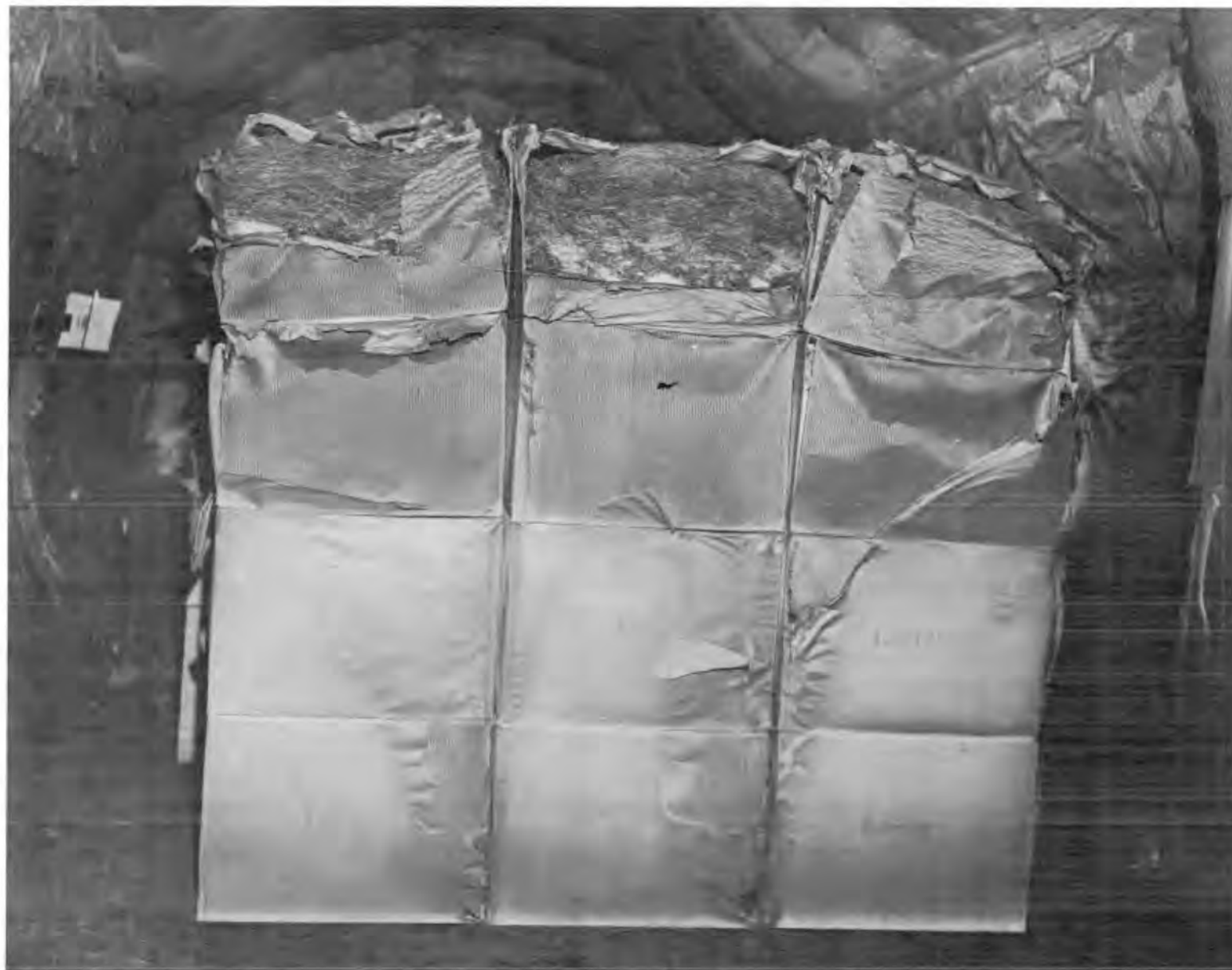
FIGURE 13 - CARGO LOADED IN CARGO COMPARTMENT IN THE 10-PERCENT CONFIGURATION AFTER AN AIRFLOW-SHUTOFF TEST, LOOKING FROM THE OULET END
