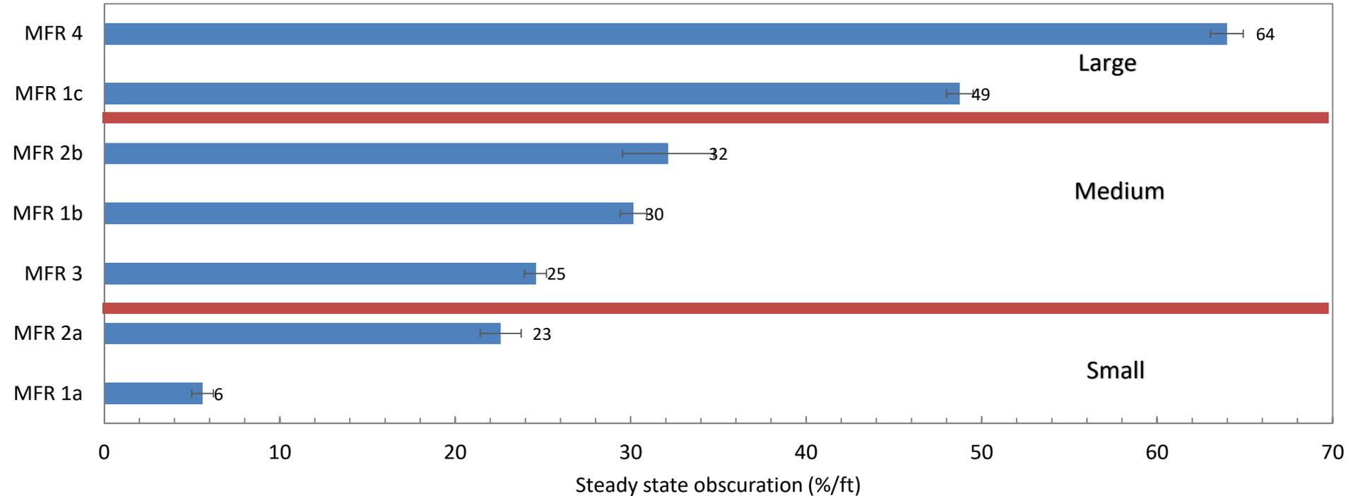
The average steady-state light obscuration of the tested aerosols was 32%/ft with a standard deviation of the means of 17%/ft
