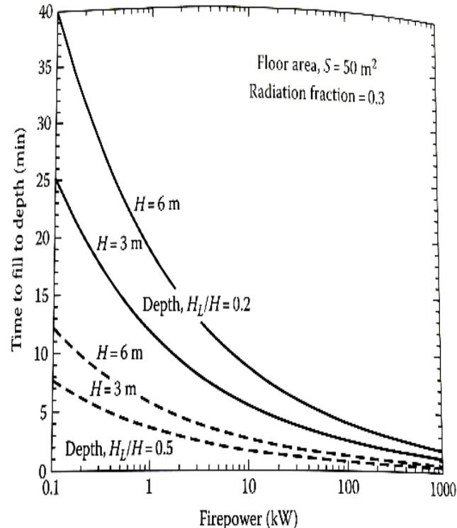
Time for smoke filling to various depth in a room heights 3 and 6 m with a floor area of  $50 \text{ m}^2$
