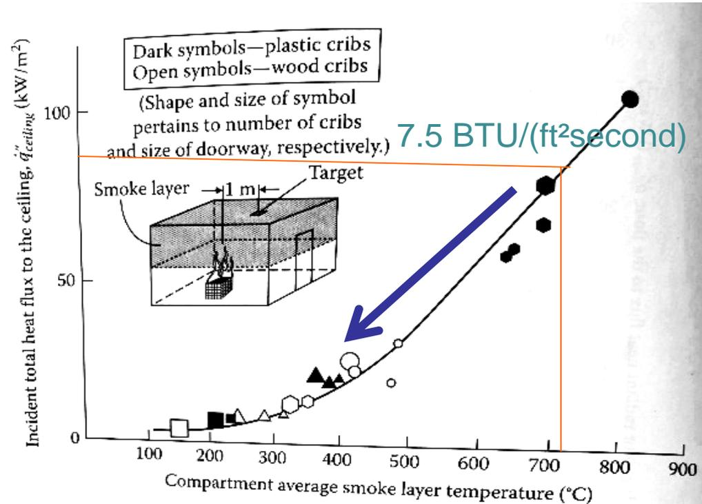
Ceiling heat flux versus compartment average smoke layer temperature
