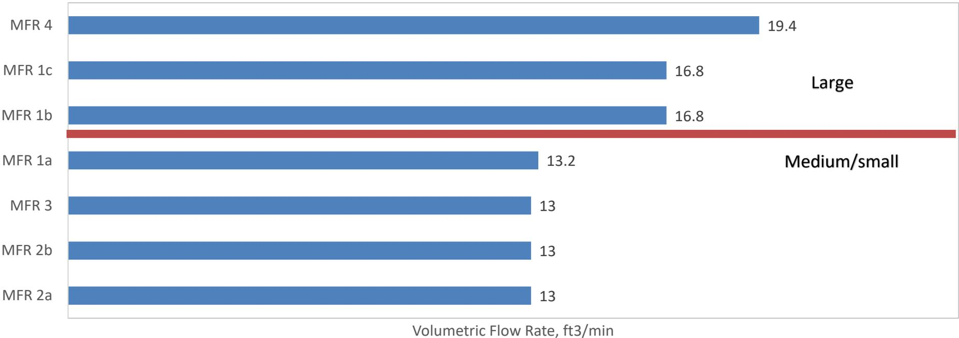
The average volumetric flow rate was 15ft<sup>3</sup>/min with a standard deviation of 2.6ft<sup>3</sup>/min
