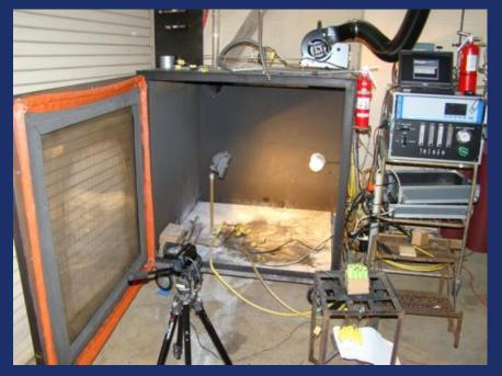
Conclusion: Halon 1301 is effective in suppressing the electrolyte fire, extinguishing the fire, and preventing any additional fire from subsequent venting. Cells will continue to vent due to the air temperature, but will not ignite in the presence of Halon 1301.
