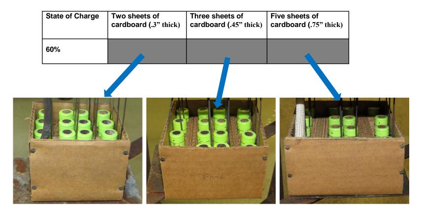
Passive Fire Protection for Lithium Battery Shipments
