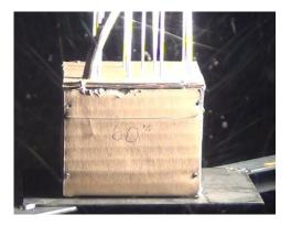
One of the 16 cells was replaced with a cartridge heater which was used to initiate thermal-runaway in the adjacent cells.
