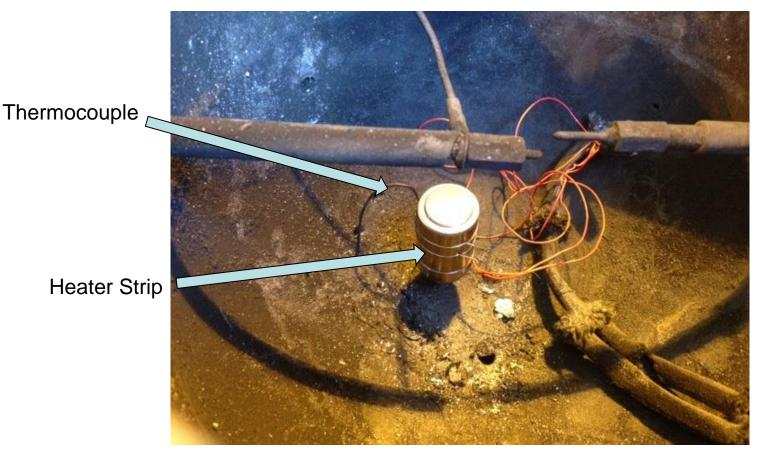
Heater Strip Capacity: 28 volts, 1.5 amps
