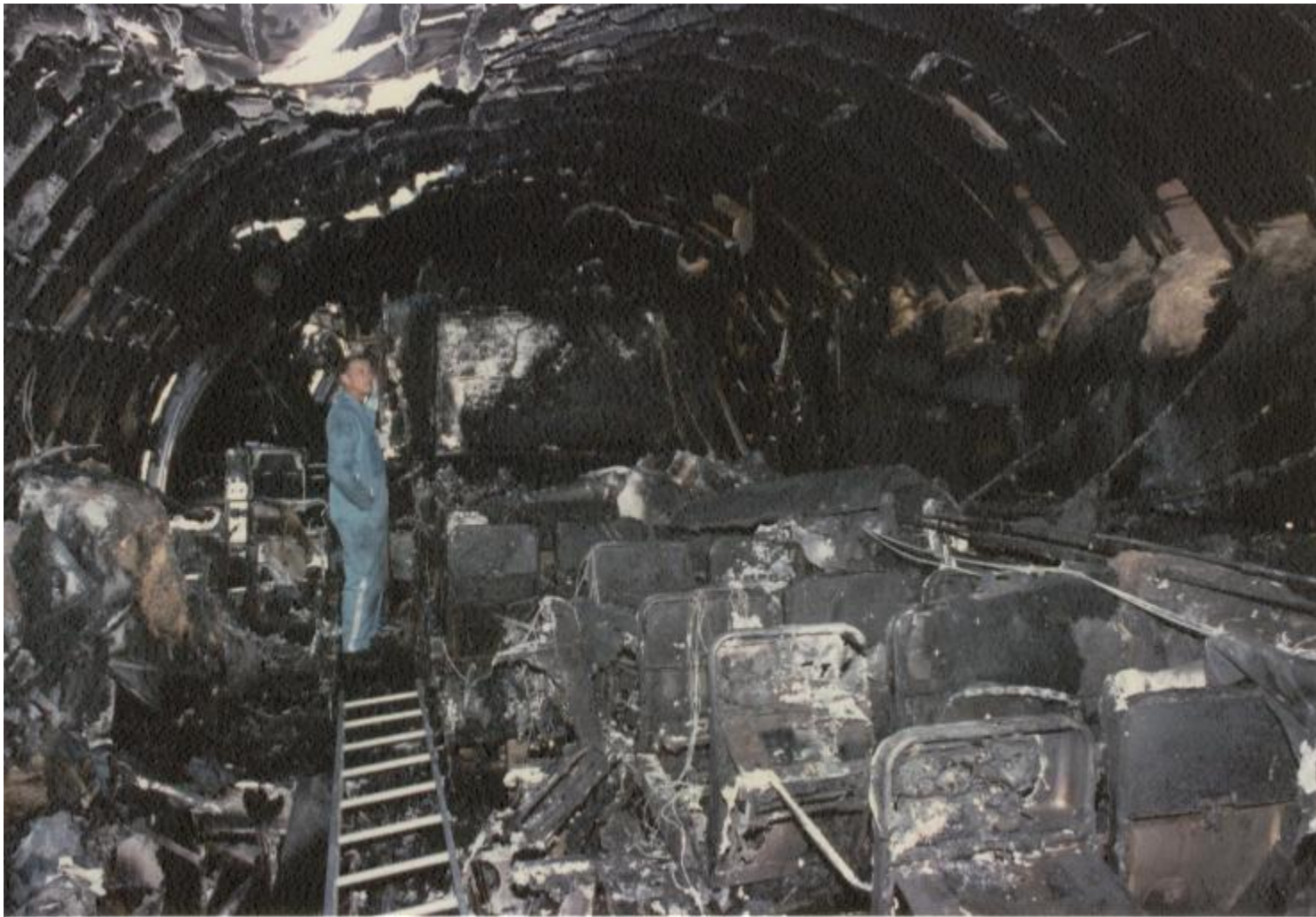
ATA DC10: Mechanic dislodged and activated O2 generator from seat back being stowed in a container in the cargo compartment
