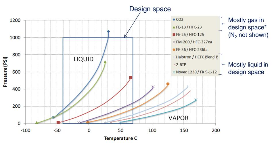
\* CO<sub>2</sub> and FE-13 may be liquid at low temperatures
