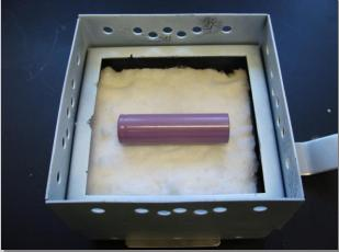
Special holder designed to prevent rocketing of cell at failure
