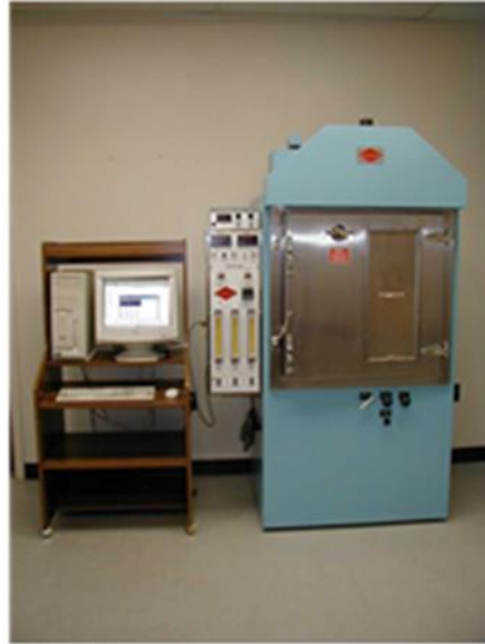
Figure 1. FAA NBS smoke emission test apparatus
