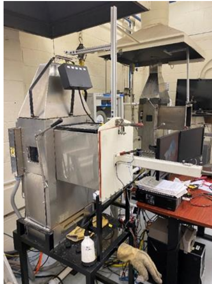
Figure 2. FAA rate of heat release test apparatus (HR2)
