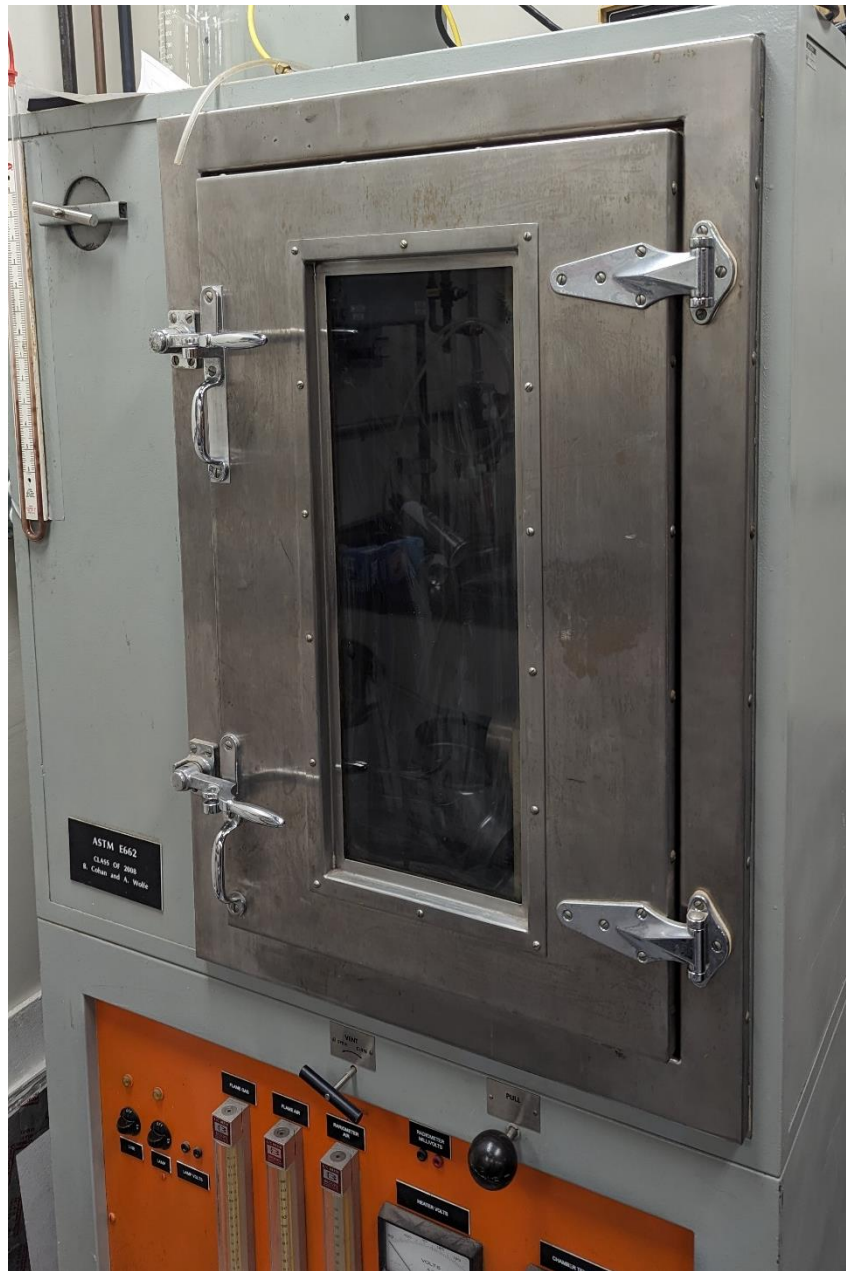
Figure 6.3 ASTM E662 chamber used for UMD tests
