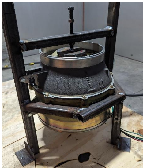
Figure 3.11 Experimental Setup for Fan Failure at the FAATC
