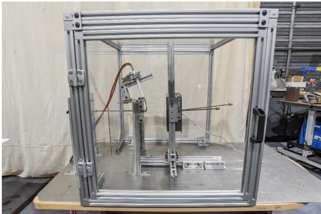
Figure 13: Burner Contained in Plexiglass Box
