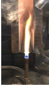
FIGURE 1. VERTICAL BUNSEN BURNER TEST
