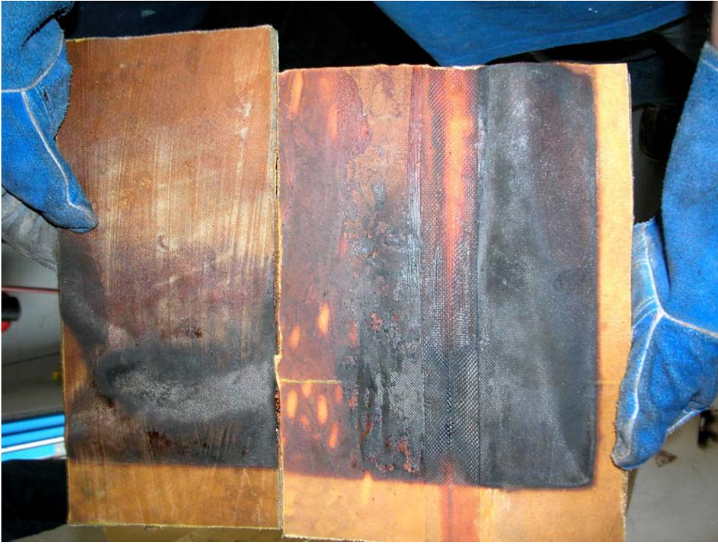
FIGURE 22. RADIANT HEAT PANEL POSTTEST DUCT CONDITION
