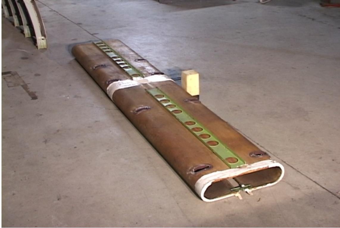
FIGURE 6. NARROW-BODY AIRCRAFT AIR CONDITIONING OVERHEAD DUCT
