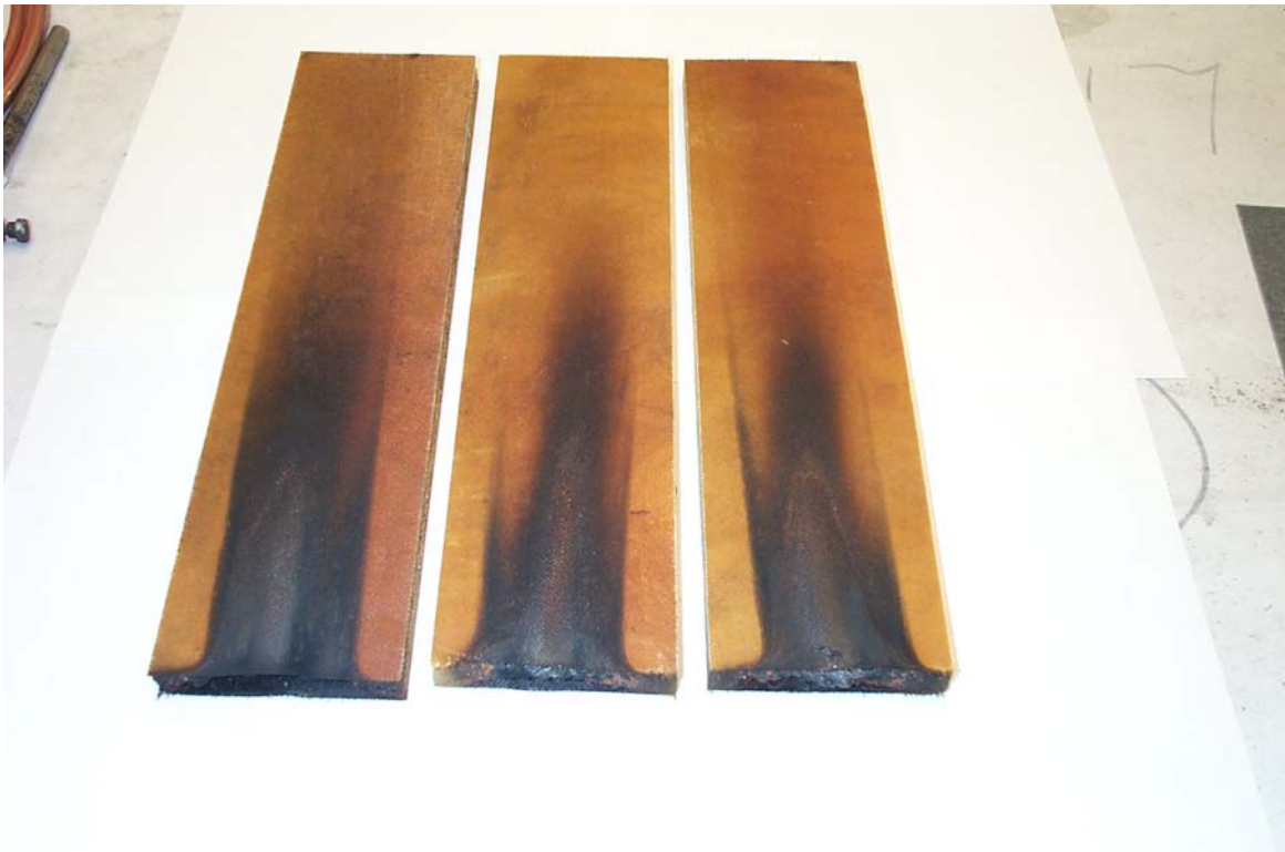
FIGURE 9. VERTICAL BUNSEN BURNER POSTTEST
