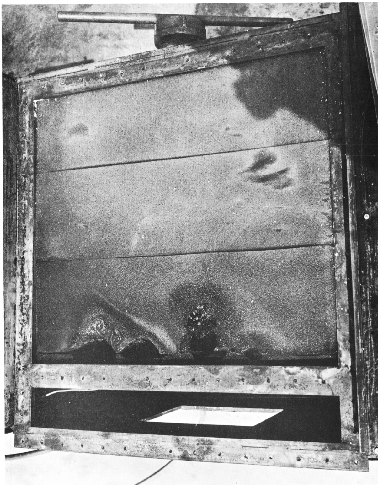
FIGURE 42 - DAMAGE TO POLYURETHANE FOAM IN TANK AREA 4" TEST ARTICLE AND JP-4
